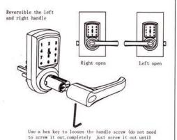
the handle can be pulled out), interchange the front
