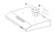
Drill the hole in the wall for the air outlet (133 mm diameter) referring to
