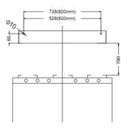
2. Now proceed with final fixing by fitting the other 2 screws. Connect a flexible exhaust duct to the hood flange, using a metal hose clamp. Tube and hose clamps are not provided.
