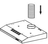
Decide on the position of the hole for the air outlet: The hole may be in the wall or the ceiling, according to your requirements, but must be in vertical line with your hood.
