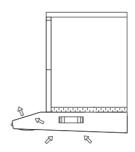
aluminum filter with carbon cotton must be replaced periodically.
