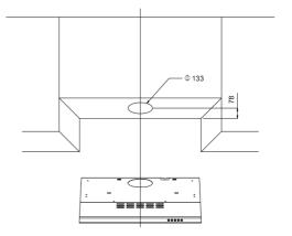
Installation is now complete. this range hood can be used either in the Ducted Mode (ducting fumes to the outside) or in the Recirculation Mode (internal recycling). We recommend you:
