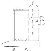
**Caution:** To reduce the risk of fire, the use of metal ductwork is preferred. Do not use flammable material to convey exhaust air.
