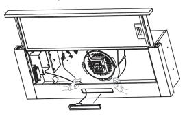
3. Take a new lamp, put it in the lamp hole of the lamp board. Gently push it back to the lamp board with your thumb. Connect the lamp wire according to the wiring
