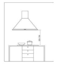
1. First, determine a good position to mount the range hood. Fix the mounting bracket to the wall with (4)ST5\*45 screws and (4)plastic expansion pipes. There should be a socket inside the mounting bracket to connect the power cord.
